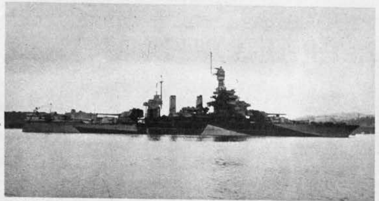
MODERN CONTROL TOWER REPLACES CAGE MAINMAST OF COLORADO
